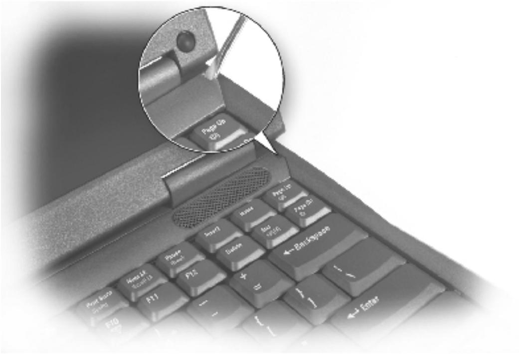
5. To release the keyboard from the palm rest, use a small, flat-blade screwdriver or plastic scribe to pull up on the right edge of the blank key on the keyboard.
